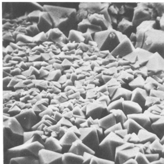
Figure 1 Cubic As_2O_3 crystals, × 1327.
